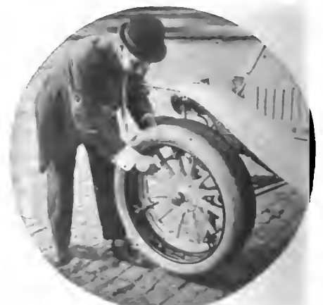
Fig. 3—Final operation, tightening nuts at ends of steel arms
